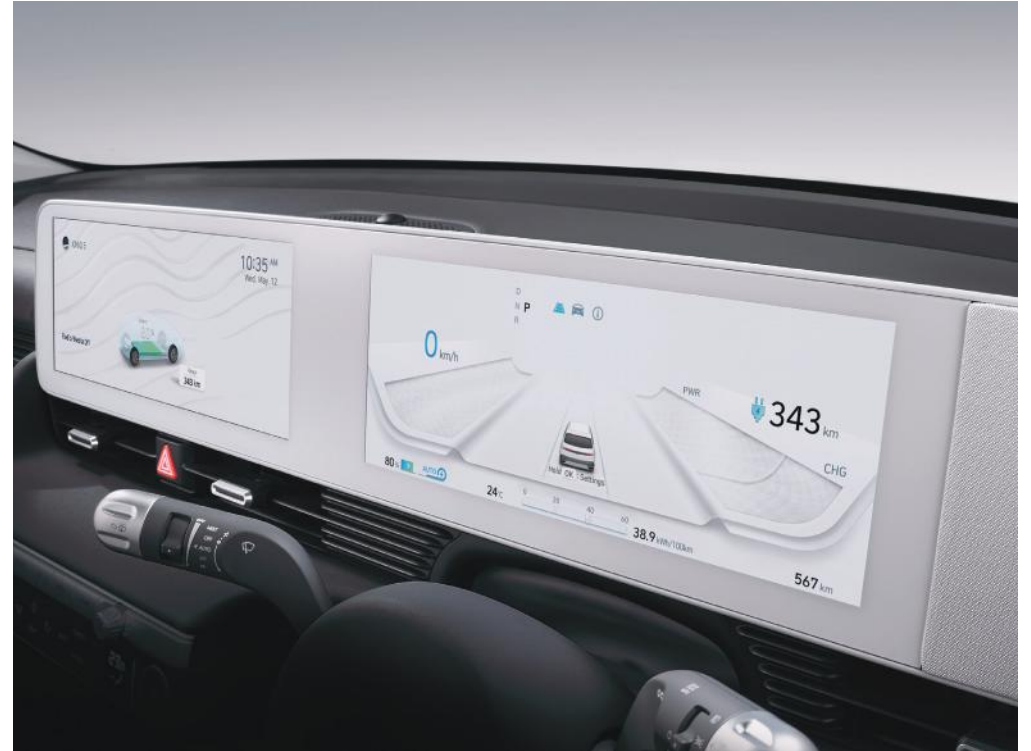
12.3" TFT LCD Cluster with integrated A/V System
