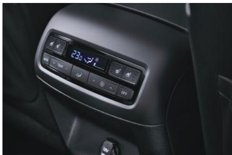
Rear automatic climate control
